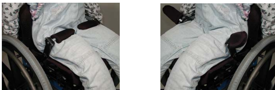
Figures 1a and 1b Rigid pelvic stabilizer on child's wheelchair: in closed and open position
